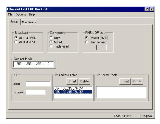
Enter Address Conversion type, FINS UDP port number and Sub-net Mask. Edit the IP Address Table: the computer where Omron Ethernet DAServer is running must be added to the IP Address Table. To add it, press "Insert" button. The "Insert Router's IP Address" dialog box appears:
